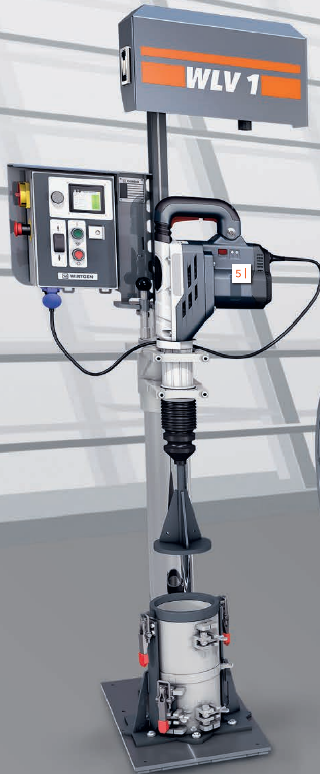
WIRTGEN WLV 1 laboratory compactor
